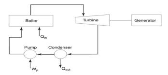
The schematic diagram also shows heat  $(Q_{in})$  being supplied to the boiler and generator connected to the turbine for the production of electricity. Heat  $(Q_{out})$  is removed by the condenser and the pump supplies energy (Wp) to the feedwater in the form of a pressure increment to allow it to flow through the boiler.
